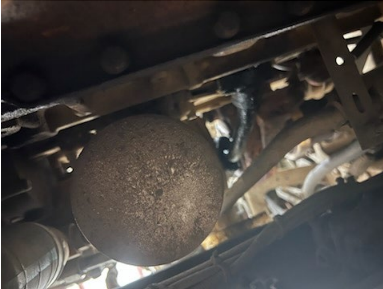
Turbo Drain Line Leak
