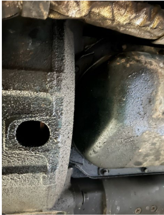
Oil Pan Leak
