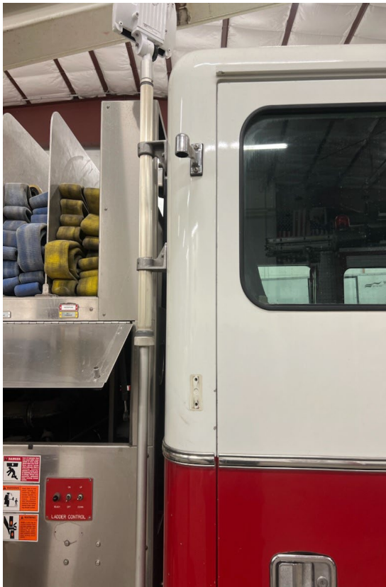
Missing Grab Handle
