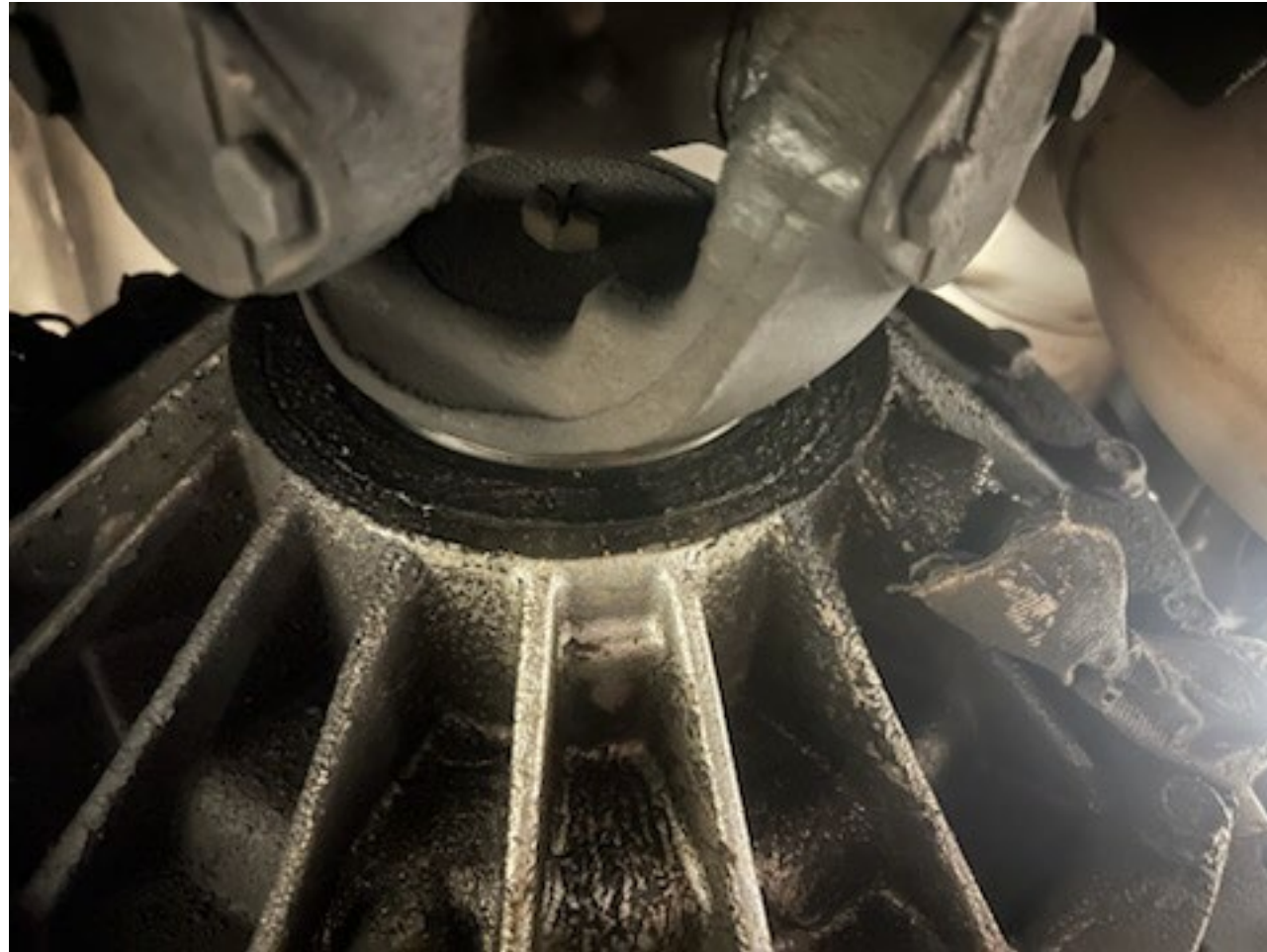
Trans Output Seal Leak
