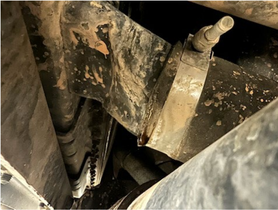
Coolant Leak at Hose
