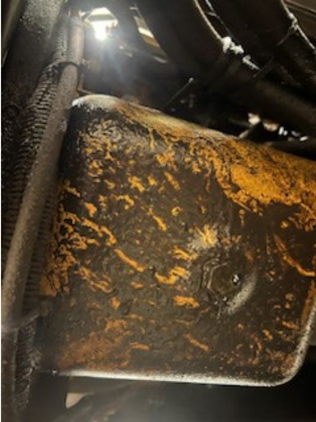
Oil Pan Leak
