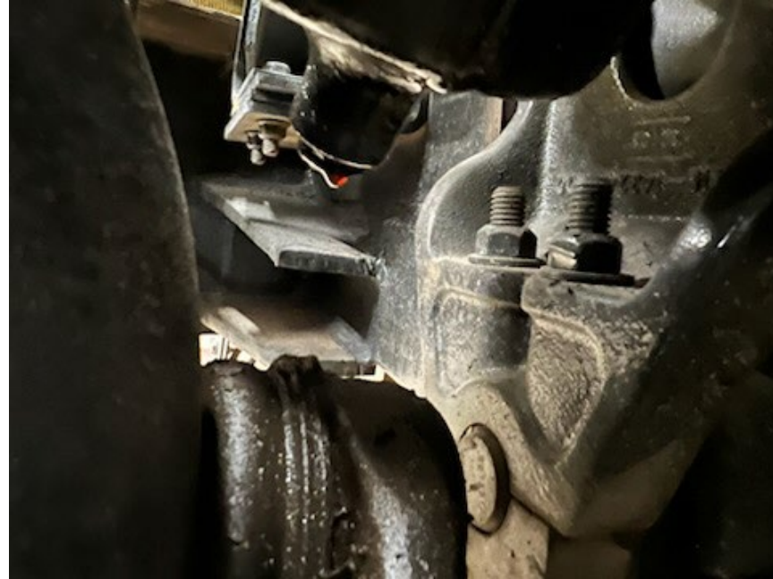
Leak at Power Steering Box
