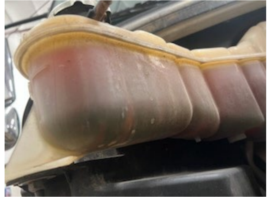
Sludge in Red Surge Tank
